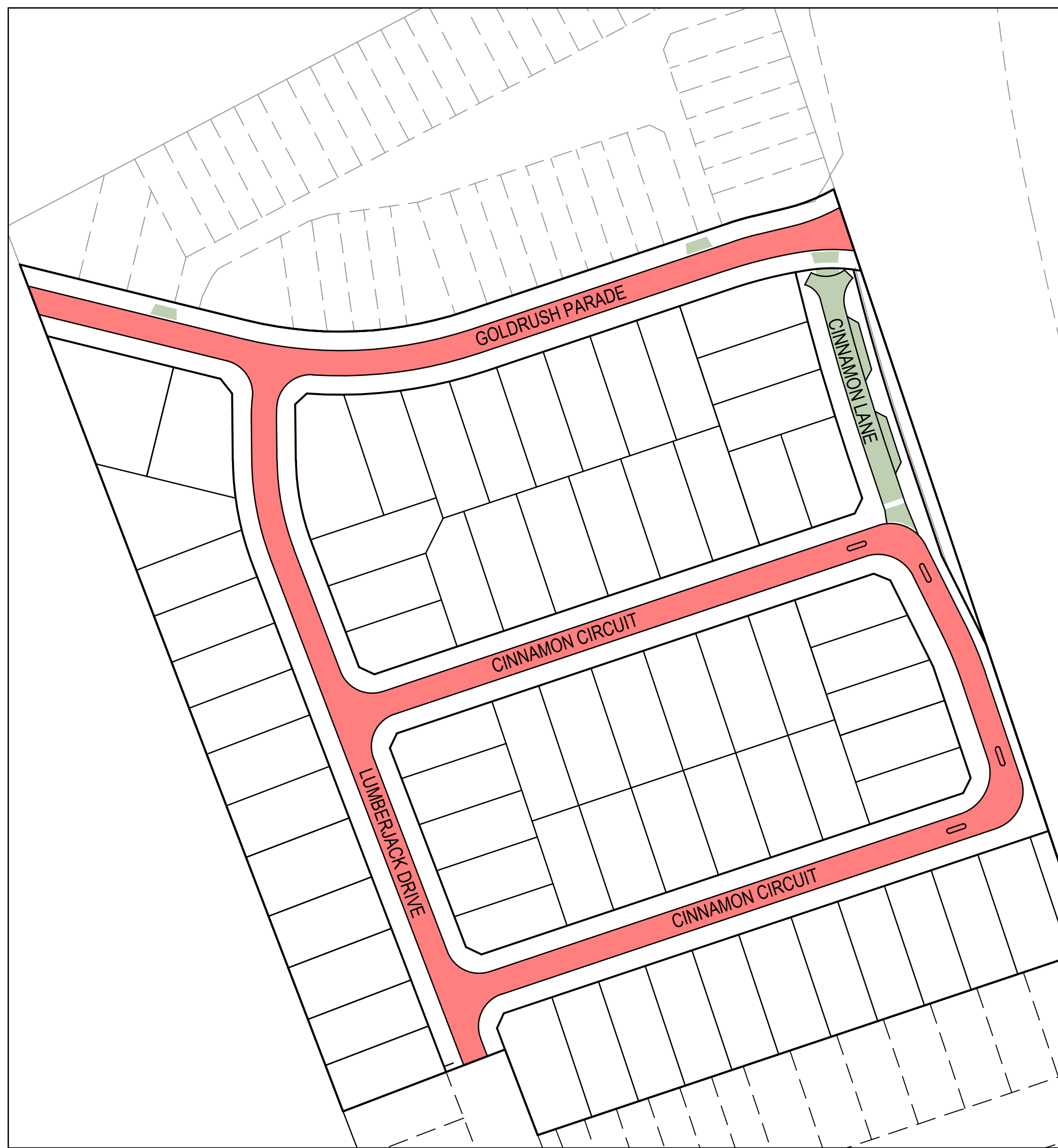
CINNAMON LANE PAVEMENT COMPOSITION 300mm PAVEMENT (EXCLUDING CONSTRUCTION LAYER)
